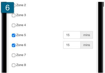
Select **Zones**. The edit box will only appear if you check the zone box. Add **Run Times** using the up arrows in the box. When finished here, select **Next**.
