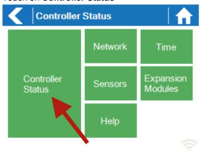
3. The serial number is shown on this screen. Note that the serial number only contains the letters **A through F** and the numbers **0 through 9**.
