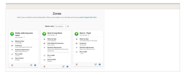
Initially, there is no master valve configured and all zones on the controller can be used as normal zone valves. To select a master valve, select the relevant zone from the list next to the text which says Master valve.
