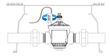
If the sprinklers turn on by manually twisting the solenoid, follow the next step to check for proper voltage.
