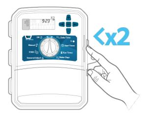
7. WAND's Wi-Fi status LED will blink amber twice per second. SAP will appear on the controller LCD.
