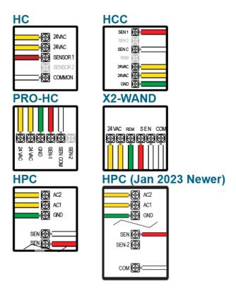
**NOTE:** HPC Controllers with date codes of JAN 2023 and newer include two sensor inputs. The SEN-SEN terminals from the original HPC Controllers have been split into SEN and SEN 2 to allow for two separate sensor installations (i.e., flow meter + rain sensor). Sensors now wire separately across the Common terminal (COM).
