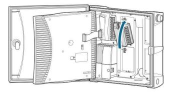
**STEP 4:** Flip the locking lever into the horizontal locked position.
