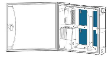
**STEP 2:** Flip the blue locking lever into the vertical unlocked position.
