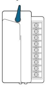
**STEP 3:** Tip the two tabs on one end of the module into the mating holes in one end of the slot, and tip the module firmly into place.
