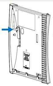
Step 4: Route antenna cable through the channel at the bottom of the facepack.
