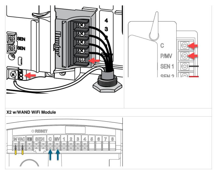
**NOTE:** With an HC Hydrawise controller, any one of your 6 or 12 zones can be configured to act as the pump start relay. We usually recommend wiring to the last zone that is not being used in the controller.
