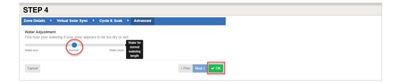
After Virtual Solar Sync has been installed and programmed, it is recommended to allow the system to run for a few days at the initial setting. Because of the variety in site conditions, the initial setting may require adjustment in order to achieve the desired performance.
