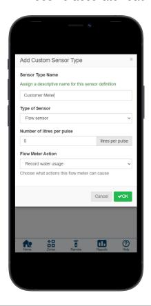
**NOTE:** For our system to detect the correct flow data and reflect it on your **Dashboard** reports, any third-party flow meter used must be a true pulse flow meter or have a reed switch. We aim for a minimum of 10 pulses per min and a maximum of 120 pulses per min. That means if the flow rate was 10 gal per min, 1 pulse per gallon needs to be set.
