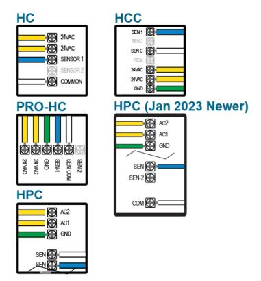
**NOTE:** HPC Controllers with date codes of JAN 2023 and newer include two sensor inputs. The SEN-SEN terminals from the original HPC Controllers have been split into SEN and SEN 2 to allow for two separate sensor installations (i.e., flow meter + rain sensor). Sensors now wire separately across the Common terminal (COM).
